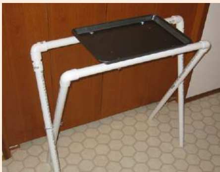
PIPE DREAMS: PVC PIPE AND A BAKING TRAY FORM THIS ACCESSIBLE TABLE.
